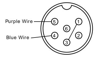
This view is looking into the socket on the back of the VIC20, and the back of the loopback connector.
